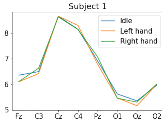
Figure 2 In this graph the signals after the logvar transformation are shown. They are averaged over all samples with the same label. As one can see, it is hard to differentiate between different types of signals due to the different sensitivities and biases of different electrodes.
