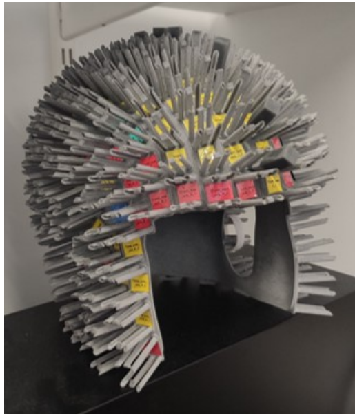
Figure 9 The MRI-fitted helmet used in the experiment. The helmet has many slots, giving the experimenter the freedom to choose where to place the electrodes.
