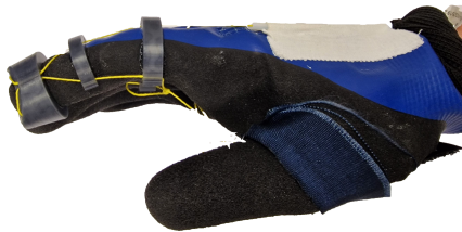
Figure 5 The second prototype, where two rings and a fingertip cover were 3D printed. They have holes, where tubes were inserted and the wires (yellow) are led through.
