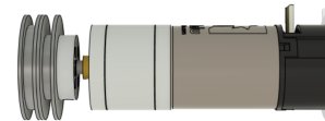
Figure 3 A 12V DC motor with encoder is used with two connected pulleys on left side. The one with the larger radius is connected to the inner side of the exoskeleton and the other pulley is connected with the outer side. The different sizes were chosen, since both sides have different differences of distance between flexion and extension.
